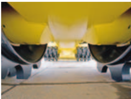
Smooth undercarriage fully protects drive components.
