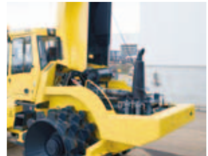
Efficient component access from the vertically opening hood.
