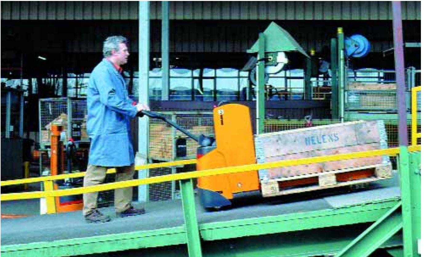
The EGU is a true professional on ramps, as even after releasing the drive switch, it "sticks" to the slope in practically all situations – and therefore there is no roll-back.
