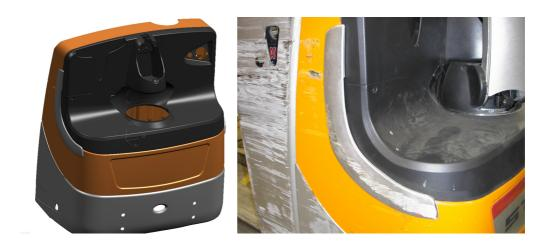
We have received several complaints about damaged or torn off motor covers on EXU – trucks and we have decided to set up in series a metallic protection.
