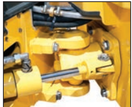
Maintenance free bolt on articulated and oscillating joint.
