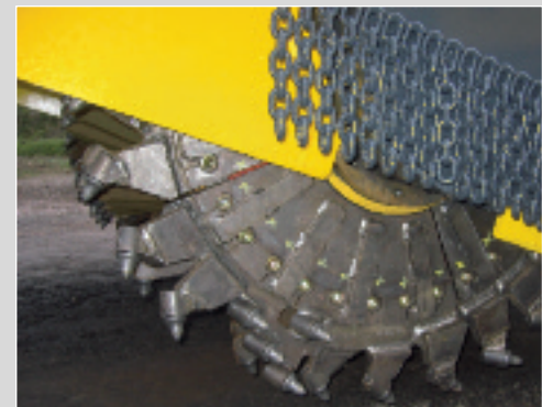
Universal rotor with individual bolt-on replaceable end segments
