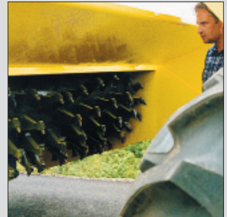
Quick replacement of cutting teeth without the need for special tools.
