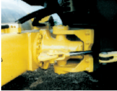
Maintenance-free, rugged, oscillating-articulation joint bolted on the outside of the front and rear frames.
