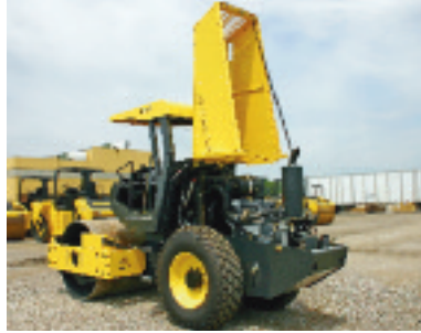
Easy access due to the vertical opening hood makes daily checks simple and efficient.
