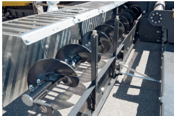
400 mm auger made of wear-resistant cast iron – BF 700 C-2.
