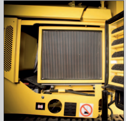
The engine compartment is accessible from three sides. This shows the generously dimensioned cooler.
