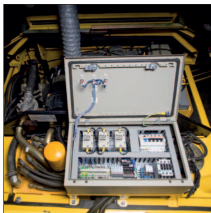
The machine control system is easy to reach in a central, enclosed control cabinet.
