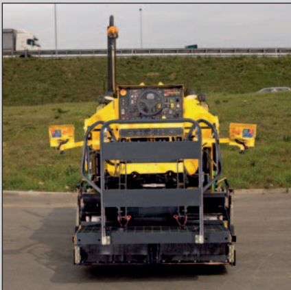
Free-positioning side-mounted metal operator stations with individually replaceable controls.
