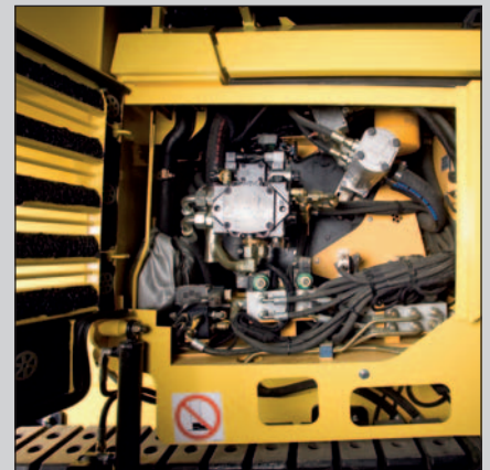
Easily accessible central hydraulics – pumps, valves, connections, etc. are all immediately to hand.
