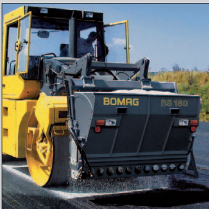
Precision chip spreader: The BS 180 distributes chips evenly and precisely.
