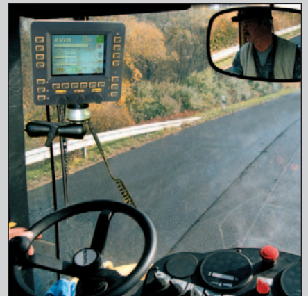
A brief glance tells all: the ASPHALT MANAGER display shows key compaction information.
