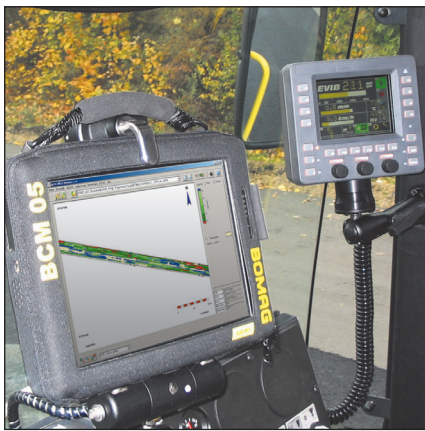
State of the art compaction technology with satellite navigation.
