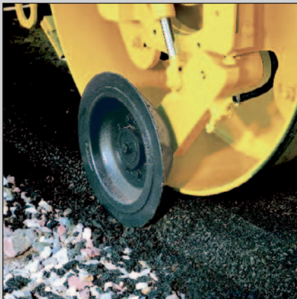
Edge compacting roll: indispensable for efficient compaction of unsupported edges.
