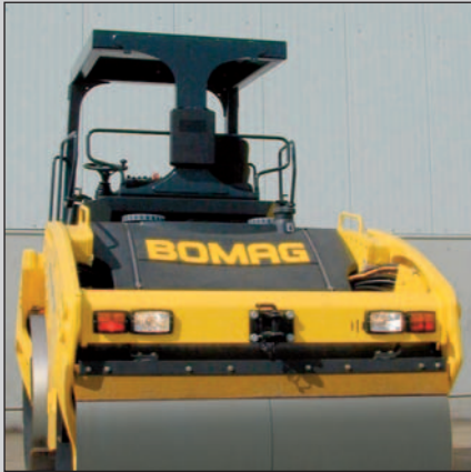
ROPS / FOPS: Optimum protection for the driver at all times.
