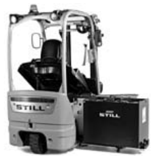
4) On-board roller platform for exchange by hoist
