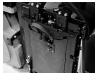
4) On-board roller platform for exchange by hoist
