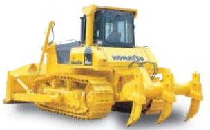
Hydrostatic Steering System (HSS) provides smooth, quick and powerful control in various ground conditions. See page 5.
