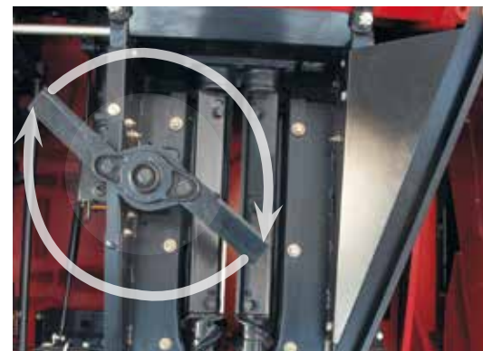
All exiting straw from the rollers is chopped
