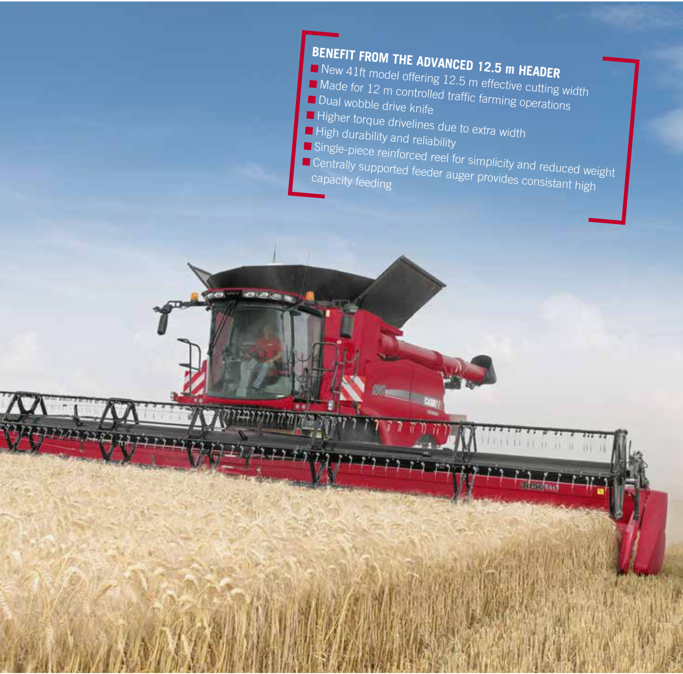
Fully hydraulically variable knife position - controlled from the cab up to 575 mm on the move
