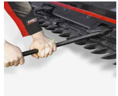
Easy servicing of the central knife drive
