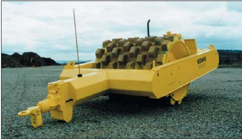
BW 6 S with towing hitch (optional equipment)
