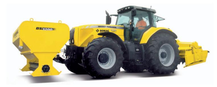
With a payload of 3,200 kg the BOMAG spreader is designed for small and medium-sized work and areas with difficult access. The 2,500 millimetre wide rotor ensures uniform spread of binder. The metering system is driven by the carrier unit's hydraulics. The hydraulic motor for the rotor can be progressively adjusted by an oil flow control valve on the tractor.
