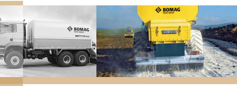
Soil stabilisation and cold recycling have long been accepted as economical and environmentally friendly methods of converting weak soils into stable foundations, and for renewing road bases while saving resources. The addition of hydraulic binders has been proven especially on difficult materials.
