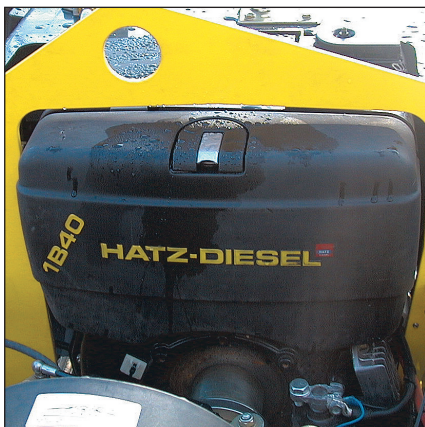
To provide the increased power needed for use with a hydraulic breaker model BW71EHB-2 is fitted with the Hatz 1 B 40 diesel engine.
