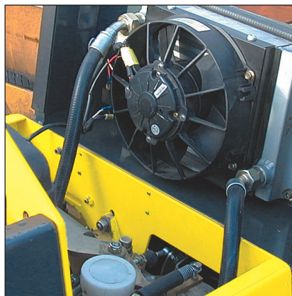
For longer life and continuous operation under high loads the roller-breaker is equipped with an additional oil cooler.
