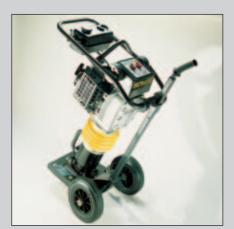
Transport trolley option for simple, rapid transport on site.
