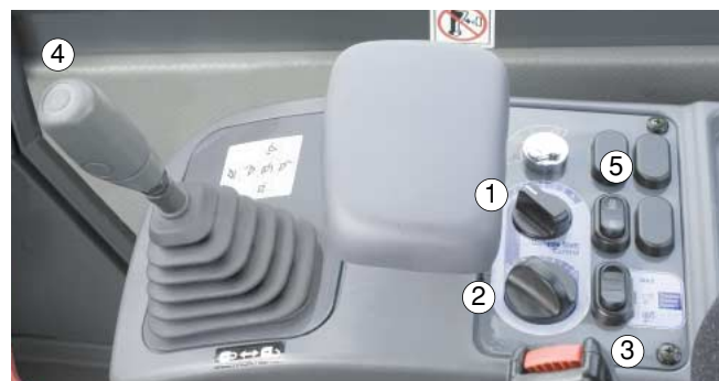
1:Speed range selector switch 2:Variable shift switch 3:Traction control switch 4:Max. traction switch 5:Fan reverse switch
