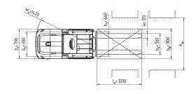
Single lift mast 2000/2500 with auxiliary lift
