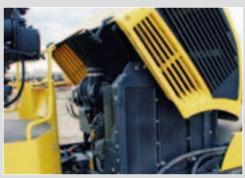
Vertical side by side coolers allow easy access for quick cleaning.
