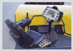
Joystick control travel direction, speed, steering, manual vibration on/off and control actuation from either seating position.
