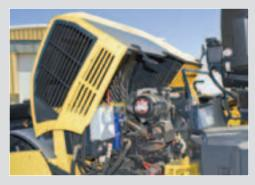
Easy opening, single hood, allows service with your feet on the ground.
