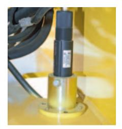
The Asphalt Mat Temperature Sensing System's on-the-go measuring of the material temperature is critical for Super Pave projects
