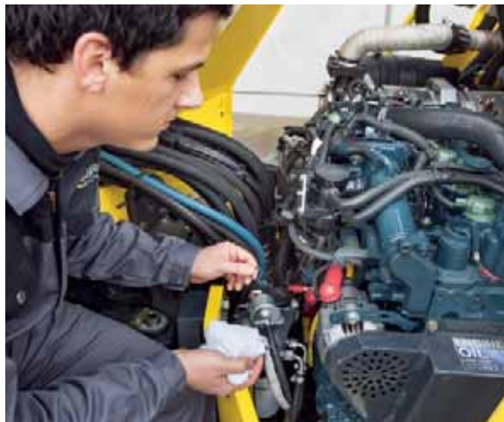
Oil level check.
