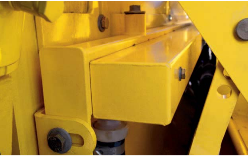
Spray bar with self-cleaning feature.
