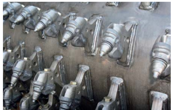
New BOMAG BRS 05 quick-change holder system.
