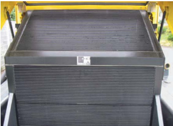
Large volume cooler with extra cooling reserves.
