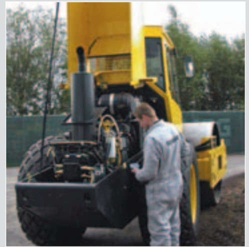
Large steel engine hood provides easy access to all service and maintenance points
