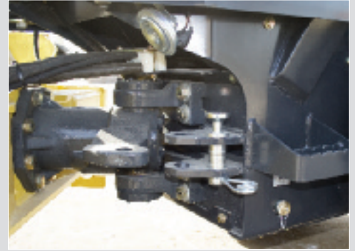
Bolt-on centerjoint is maintenance-free
