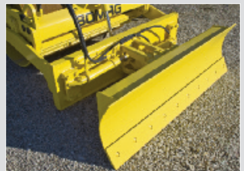
Optional angle blade enhances machine versatility
