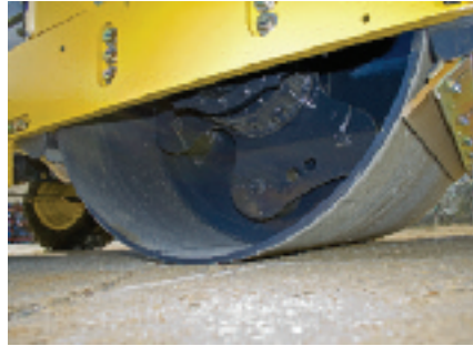
Scrapers are positioned at both the front and rear of the drum to ensure a clean drum surface
