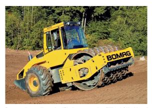
Power and versatility on landfill site construction: BW 213 DH with pad foot shell and tractor tyres.
