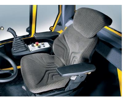
The cab provides the driver with the best all-round visibility, especially to the wheels. The generous space and well thought-out storage areas create a comfortable workplace. A standard feature of single drum rollers with cabs is the sprung deluxe seat with many adjustment options \*). The entire seat can be shifted to the side for better visibility \*\*).
