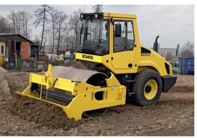
Spread and compact at the same time: Single drum roller with dozer blade, in this case a BW 177  $\rm DH-4.$
