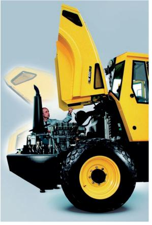
A safety feature: The small number of service points can be accessed from the ground. The hood can be easily opened by hand.
