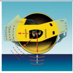
BOMAG VARIOCONTROL: linear vibration ...
