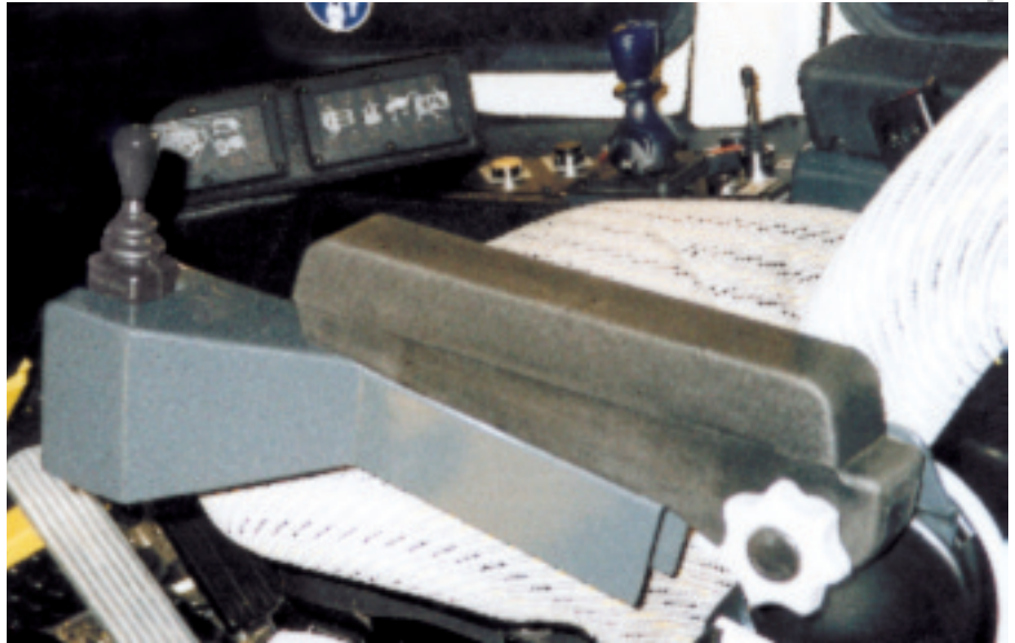
Ergonomic control layout including joystick steering control.
