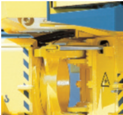
Only BOMAG has \pm 15^\circ oscillation movement between front and rear frames.
