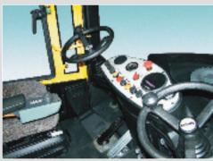
Two steering positions with a swivel/sliding seat makes the work environment more comfortable and safe
