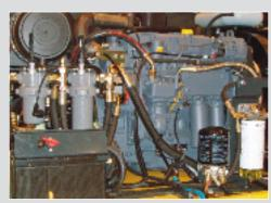
The engine: Rear, transverse positioned for ease of access and maintenance.
