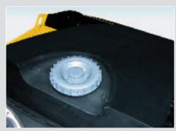
Standard pressurized waterspray produces even tire wetting – regardless of grades or water tank level.
