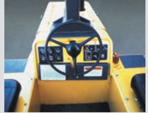
Cockpit design places controls within easy reach and provides unobstructed visibility
