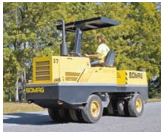
BW11RH in action on an asphalt resurfacing application
