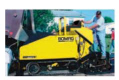
The BF4413 Machine paving a side street.
