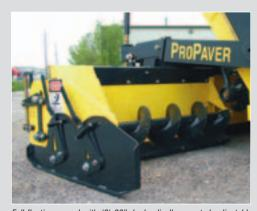
Full floating screed with (2) 30" hydraulically operated, adjustable screed extensions.
