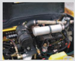
The 60 horse power Cummins diesel engine is protected by a high water temperature, low oil pressure shut down system.
