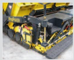
Power depth adjustment controls mat thickness.
