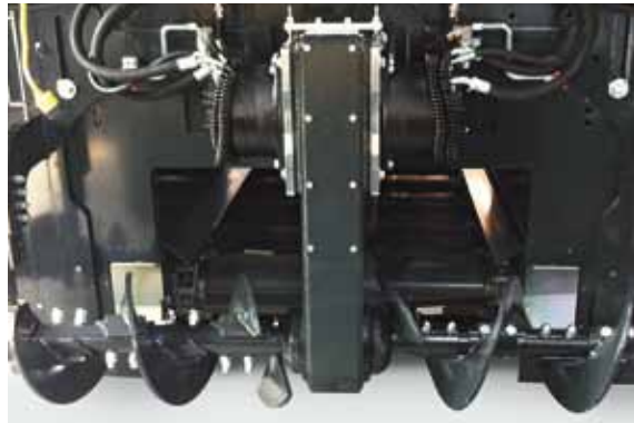
Heavy-duty drive for scraper belt and auger.
