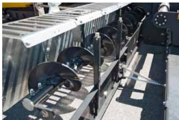
450 mm auger made of wear-resistant cast iron.
