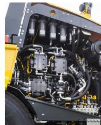
Fuel saving up to 17% - demand driven hydraulics - the BOMAG ECOMODE
