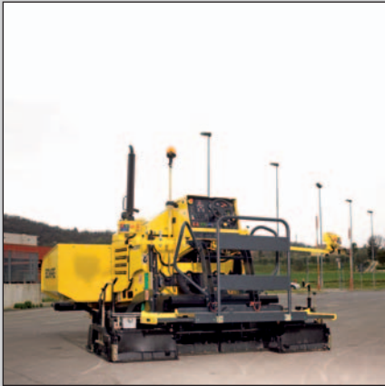
The operator's platform offers a secure, obstacle-free working place. The walk board can be adjusted to the screed width.
