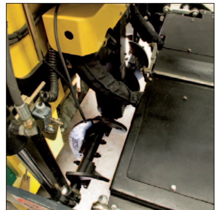
The auger can be adjusted in height mechanically – also hydraulically, on request.
