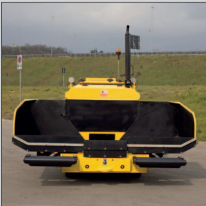
A high capacity 2.9 m hopper width, 5 tonne material capacity and adjustable push rollers ensure problem-free truck loading.
