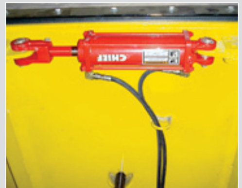
The BOMAG 3313 paver offers 3/8 inch thick hydraulically actuated hopper wings.
