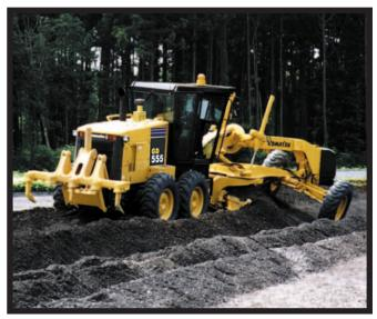
**High Performance Komatsu SAA6D102E Engine** The GD555 gets exceptional power and efficiency from the turbocharged and air to air aftercooled engine. Output is 119 kW **160 HP** SAA6D102E (variable horsepower in higher gears) providing excellent tractive effort with good fuel efficiency.
