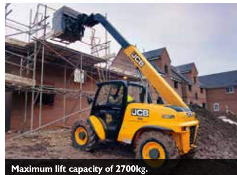
Maximum lift capacity of 2700kg.
