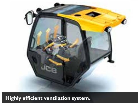
Best-in-class comfort with one of the largest cabs in the industry. The cab conforms to ROPS ISO 3471 and FOPS ISO 3449 and puts the operator firmly in control.
