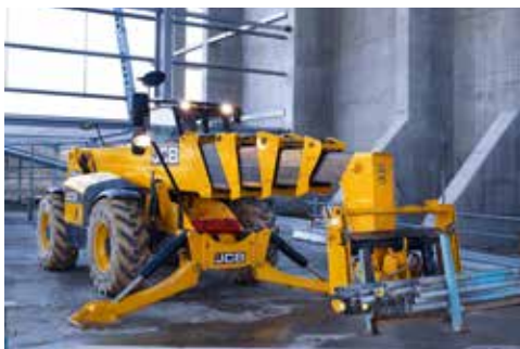
Sway chassis keeps machine level on uneven ground.
