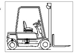
Stability is achieved by virtue of the high position of the steer axle articulation point. This means that the centrifugal force has less effect because of the short length of its lever arm from the tipping line.
