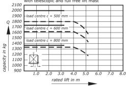
Tele up to 2240 mm Tele/full free lift from 2290 mm
