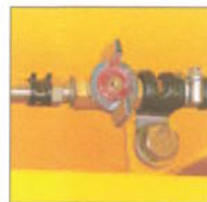
Fuel Drain Valve
