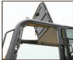
Large roof window
